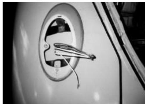
The taillights get wired just like the front end. Wires on this driver side get jumper wired over to the passenger side and to the license plate light.
