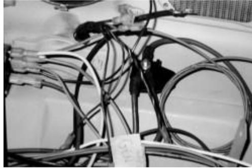
Up front again, we added new terminals to the steering column wires...
