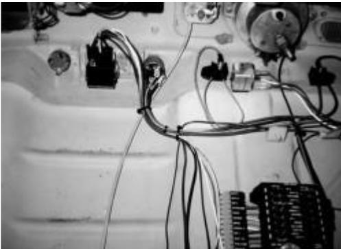
Installed in its new location, the headlight switch wires get routed to the right places.
