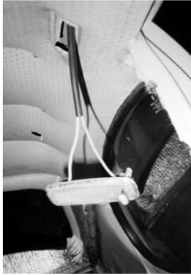
Don't forget the dome light. We put these wires inside some heavy wall shrink tubing and used the old wires to pull the new wires through the body.
