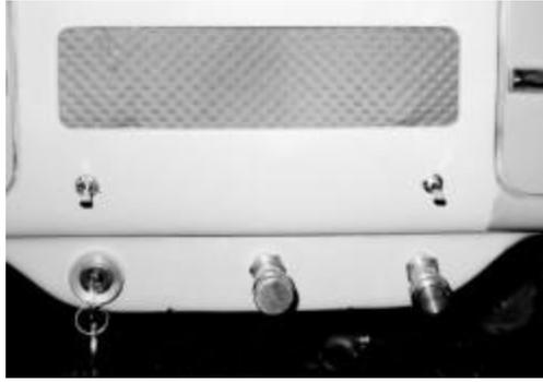
Here is our new switch grouping - ignition, headlights and wiper switches on the bottom; the toggle over the ignition is for 4-ways and the one over the wiper is for the electrical windshield washer.
