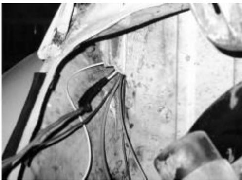
Running the wiring to the back end, we found that a left over piece of the heavy 10 gauge primary battery feed wire came in handy. We fished it through the body easier than small wires and then pulled the whole bunch in one shot.
