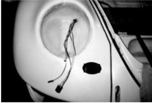
We can then run and terminate the headlight wires with the sockets provided in the kit. The individual lead is for the parking light that is in the headlight assembly.
