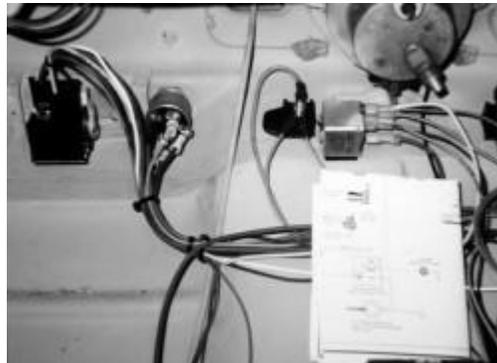
One of the replacement/upgrades we are doing is to replace the old dimmer switch relay with a newer, smaller unit also from Watson's. The headlight switch feeds the relay, which is then triggered by the stock grounding switch in the turn signal arm.
