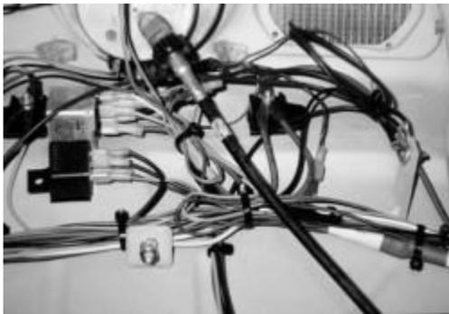
All of those tie-wraps that come in the kit help to clean up the wiring. On the right of the photo you can see our master ground connection attached to the old flasher relay mount.
