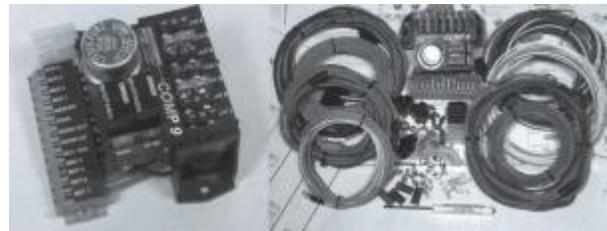
can get add-on's like the ones shown on this page that have individual inputs for each fuse so that you can choose or change the input source as needed. With any of these panels, you get extra circuits with a minimum of hassle.
